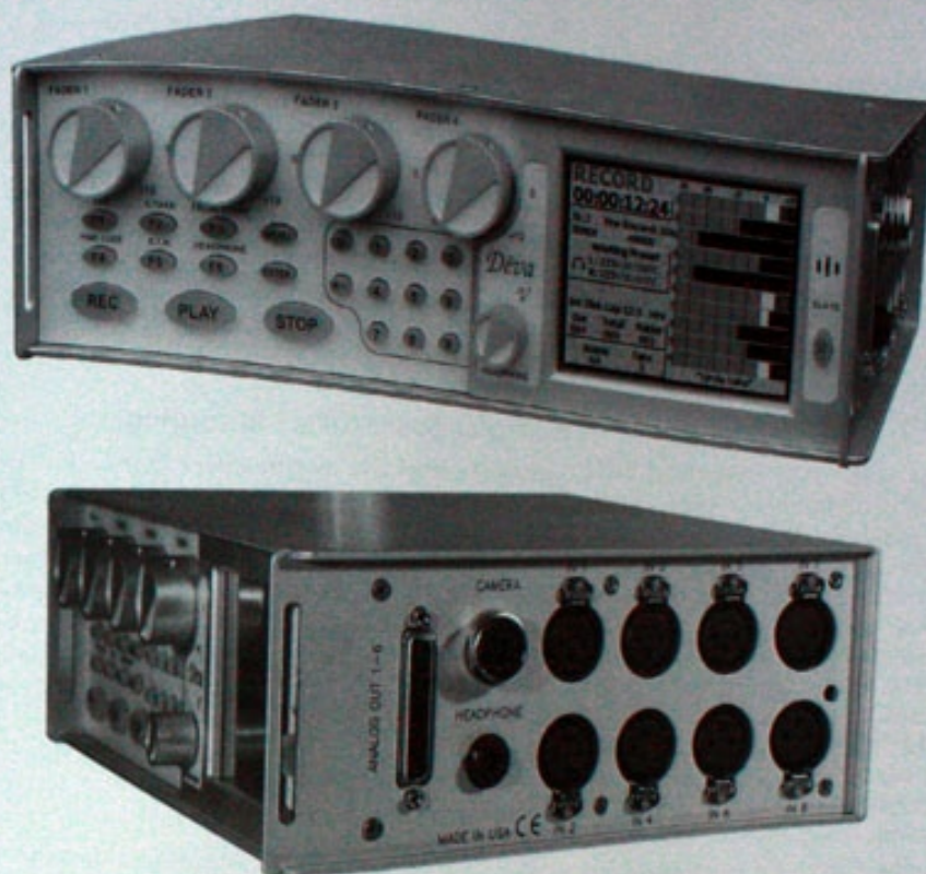
11-14 Portable hard-disk field recorder (front and right side views). This model is a multidisk (up to three disks can be recorded at the same time), multiformat recorder. It is capable of real-time 10-track, 24-bit, 192-kHz recording with 123-dB dynamic range and can deliver two disks with different sampling rates to postproduction. Among its other features are FireWire disk recording, internal 16-input and 16-bus digital mixer for surround recording, scene and take data documentation, and quick identification of takes and false starts. A fully charged battery has a three-hour running time.
